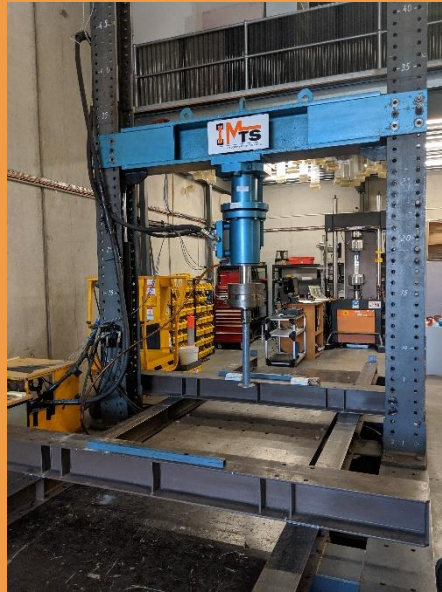
500kN (50t) Servo Hydraulic Universal Testing Machine - Tension, Compression & Fatigue
