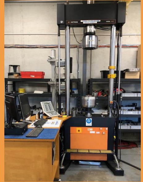
500kN (50t) Servo Hydraulic Universal Testing Machine - Tension, Compression & Fatigue
